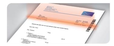
The DS-90i can read any type of coding such as OMR, 1D barcodes and 2D Datamatrix. Furthermore, the code can be printed anywhere on the document. This unique feature provides full flexibility to fullfill any layout requirement.
